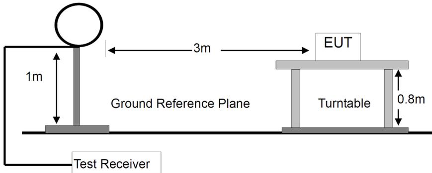
For Radiated Emission 30-1000MHz
