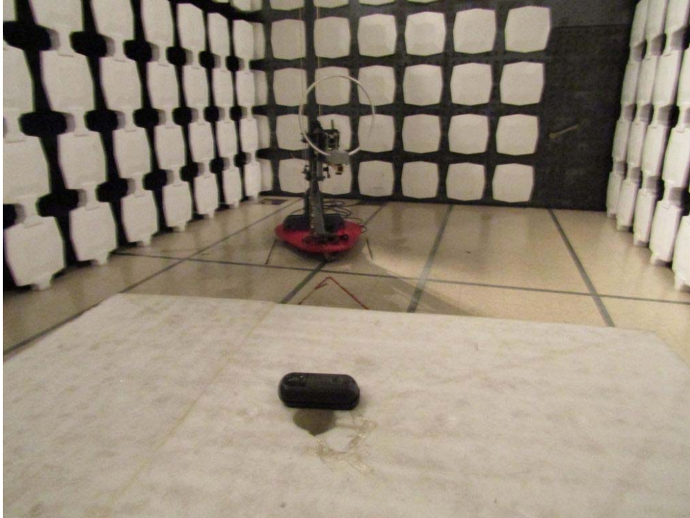
Measurement of Radiated Emission Test Set Up
