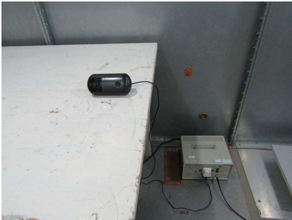
Measurement of Conducted Emission Test Set Up
