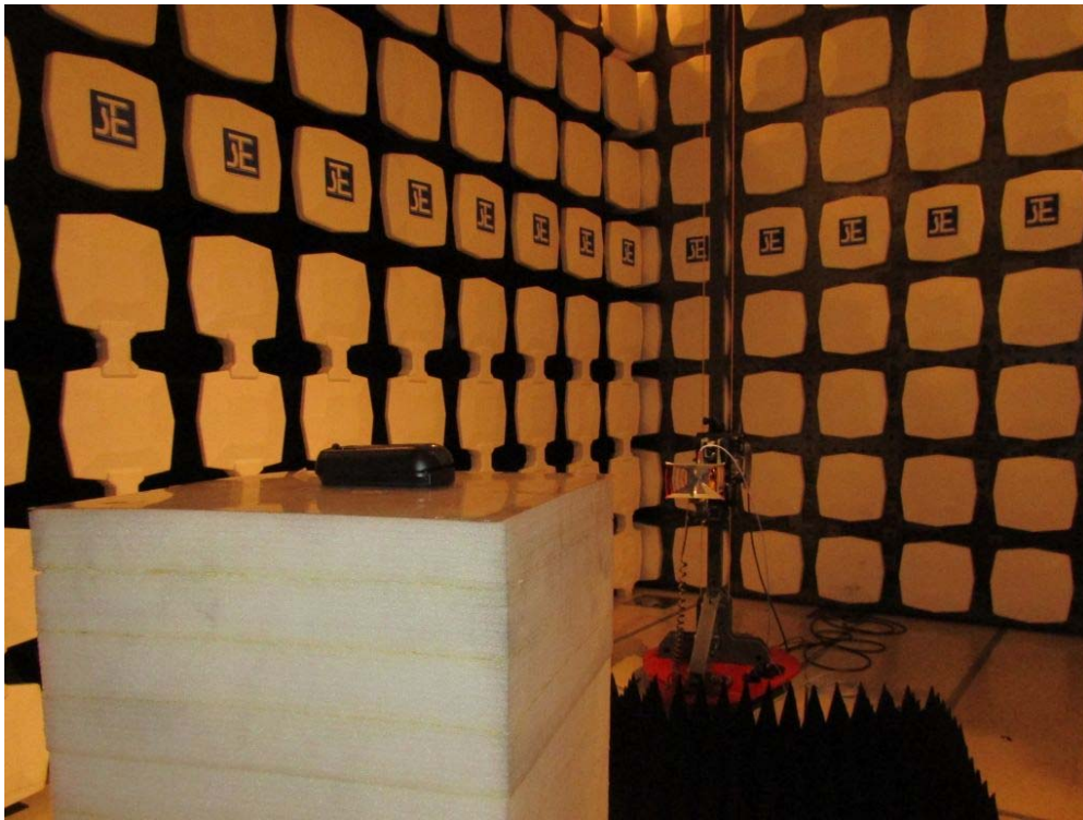
Measurement of Radiated Emission Test Set Up
