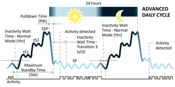
When using the Advanced Daily Cycle, the SCS™ Connect enters and leaves Standby Modes in progressive stages to save energy. At the start of each day, it leaves Standby Mode and commences a Pulldown. This continues until Transition 3 Set Point (tS3) is reached and the Inactivity Wait Time - Transition 3 (yt3) commences. During this time if any activity is detected, the Pulldown continues until the Operational Set Point (SP) is reached. When this is reached the SCS™ Connect enters the Normal Mode.
