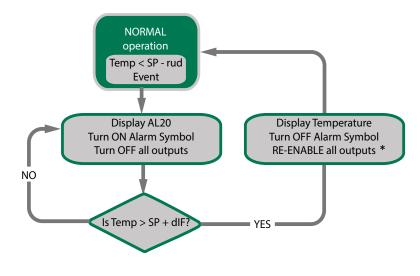
\* Compressor will not re-start unless it has been off for the minimum off time
