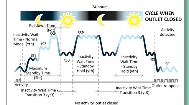
If a Retail Outlet does not open on a particular day, to save energy the system returns to full Standby. This can occur in several stages. If no activity is detected during the Inactivity Wait Time – Transition 3, the SCS™ Connect returns to Full Standby Mode, and is then ready to start the Pulldown again at the start of the next day as per normal. Should any activity be detected while in Full Standby mode, the SCS™ Connect will immediately commence a Pulldown.
