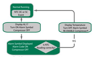
\* Compressor will not re-start unless it has been off for the minimum off time
