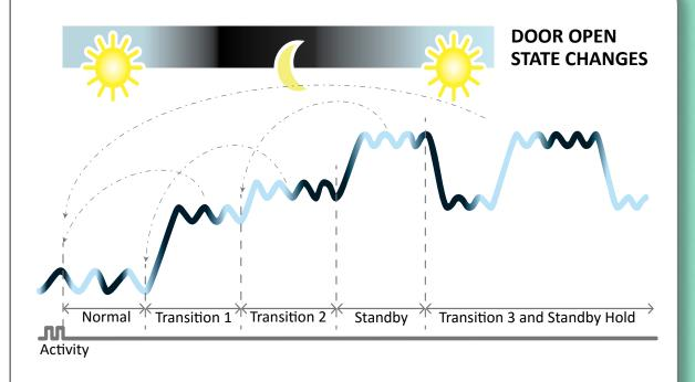
If the cooler is in Normal mode and an activity is seen, the "Inactivity Wait Timer - Normal Mode" will be reset.
