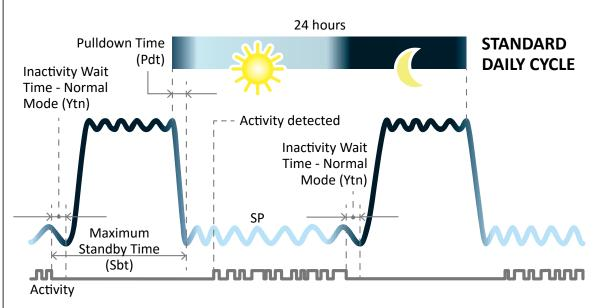
When in Non-Perishable Mode, the SCS™ Connect enters Standby Mode at night to save energy. At the start of each day, it leaves Standby Mode and commences a Pulldown. The start of the Pulldown is timed to ensure that the Operational Set Point (SP) is reached before the first customer Activity is expected. When the Operational Set Point (SP) is reached the SCS™ Connect enters Normal Mode.
