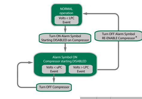
\* Compressor will not re-start unless it has been off for the minimum off time
