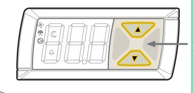
Press Up and Down Button together to enter Service Mode, followed by the 9-digit PIN code
