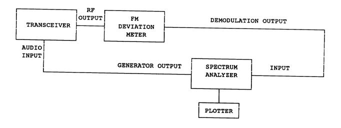
On that block diagram, the HP 3885A spectrum analyzer having the tracing generator, and the Marconi 2955A Radio Communication Test Set having an output of a demodulator, are used. After the calibration was made (the -20 dBm reading of the spectrum analyzer corresponds to the 9 kHz deviation) the spectrum analyzer was set to scan the frequency from 300 Hz to 30 kHz, with the same audio input level as described above, and with compressor OFF and expander OFF.
