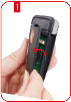
Push the slide button to separate the shell
