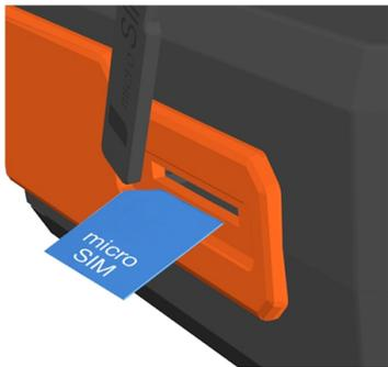
Push a SIM card into the slot as shown in the picture (make sure the circuit chip is facing down), until you hear a click and the SIM card is fixed securely in the slot.
