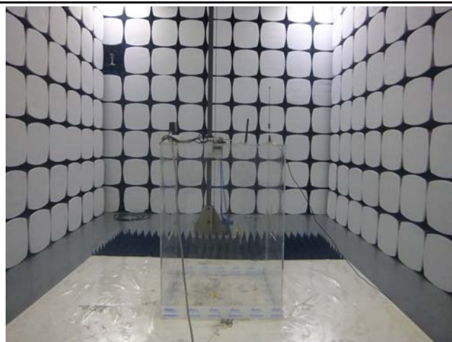
Radiated Spurious Emissions Test Setup Above 1GHz
