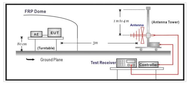
Above 1GHz Test Setup:
