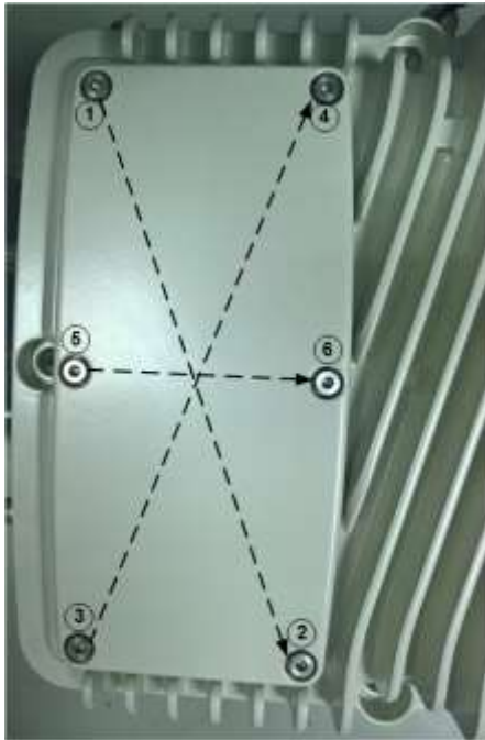
Figure 13: Screw Tightening Pattern
