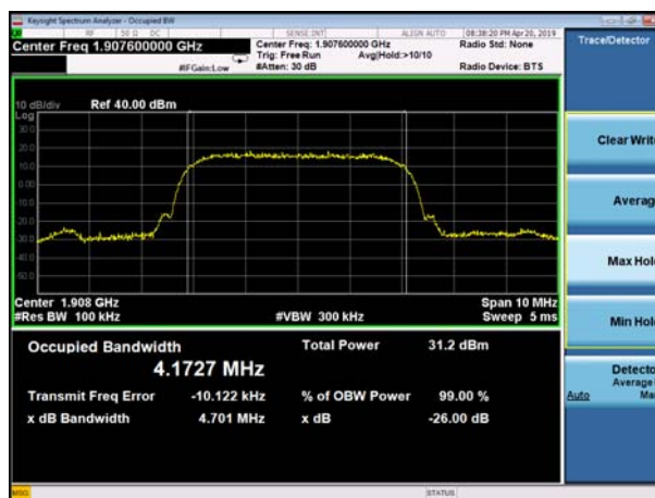
(Plot F3: WCDMA 1900MHz Channel = 9538 Occupied bandwidth)
