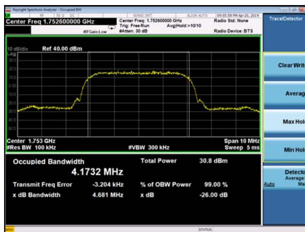
(Plot G3: WCDMA 1700MHz Channel = 1513 Occupied bandwidth)
