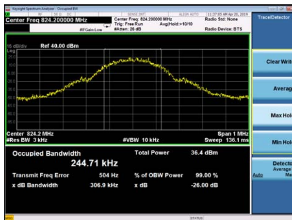
(Plot A1: GSM 850MHz Channel = 128 Occupied bandwidth)
