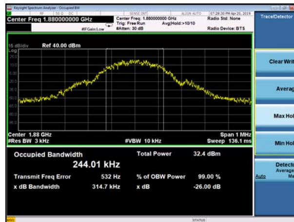
(Plot B2: GSM 1900MHz Channel = 661 Occupied bandwidth)
