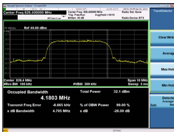
(Plot E1: WCDMA 850MHz Channel = 4132 Occupied bandwidth)
