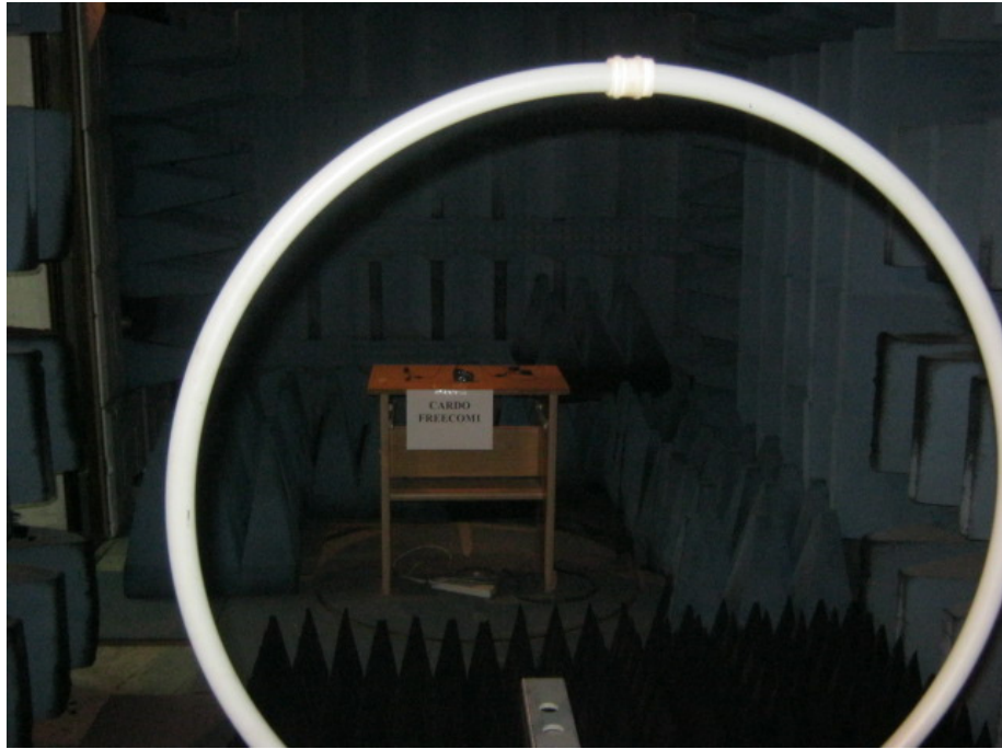
Note – Preliminary radiated emission testing set-up. All emissions were at least 20dB below the limit
