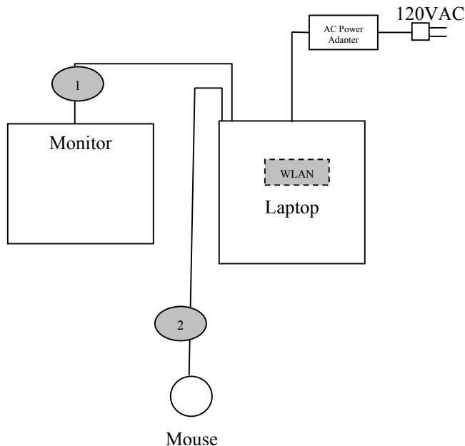
Cable 1: This is a 6-foot braid and foil shielded round cable connecting the Latitude | D410 Notebook Computer with the Dell LCD monitor. It has metallic DB-15 type connector at the computer end and is hardwired to the monitor. The cable is bundled to a length of one meter and the shield of the cable is grounded to the chassis of both devices via the connector shells.
