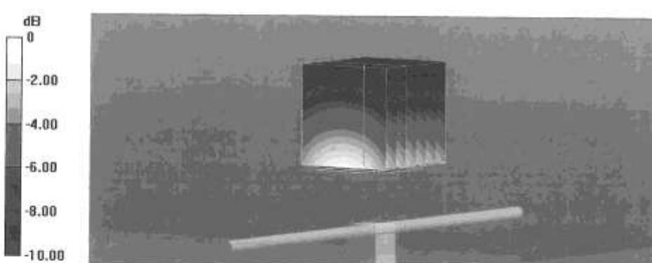
**Impedance Measurement Plot for Body TSL**
