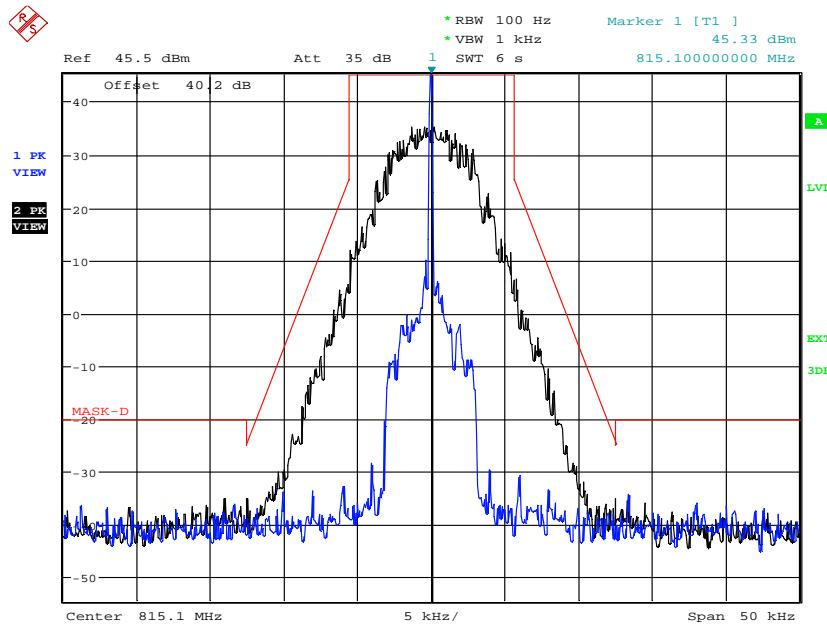
**5.8.7.16. Configuration: Mask D, Band 3: 815.1MHz, F1W, Digital, Low power FCC 90.210 & IC**
