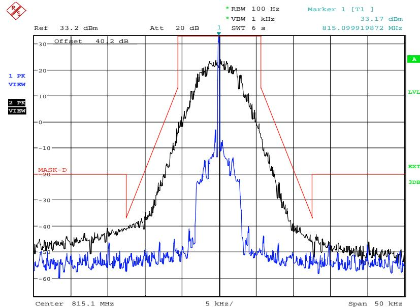
**5.8.7.17. Configuration: Mask D, Band 3: 823.9MHz, F1W, Digital, High power FCC 90.210 & IC**
