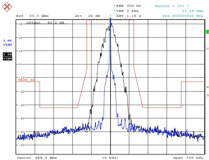
**5.8.5.29. Configuration: Mask 90.691, Sub Band 4: 854-869MHz, 860.1MHz, F1W, Digital, High power**
