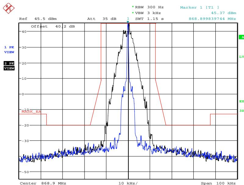
**5.8.5.28. Configuration: Mask 90.691, Sub Band 4: 854-869MHz, 868.9MHz, F1E&F1D, Digital, Low power**
