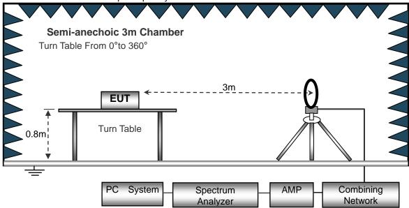
(B) Radiated Emission Test-Up Frequency 30MHz~1GHz
