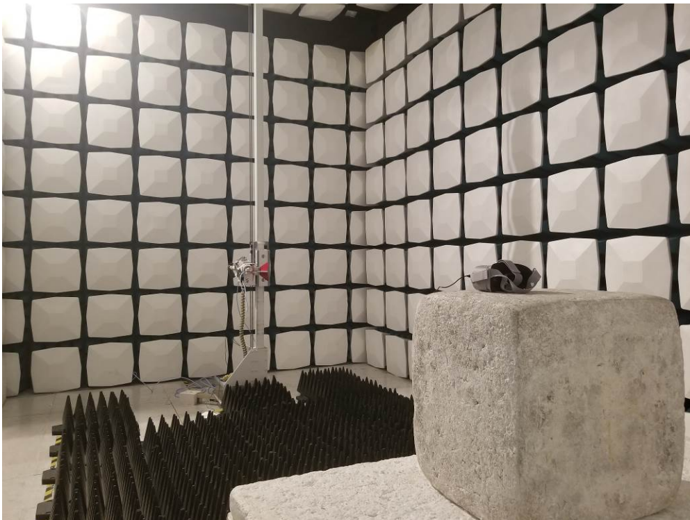
Description: Radiated Emission Test Setup for 1~18GHz
