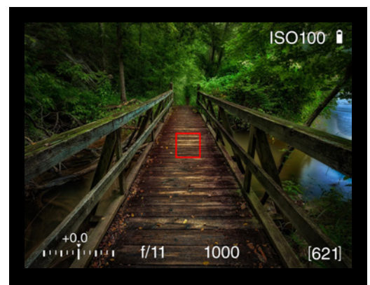
Red AF indicator. AF analysis failed to focus.
