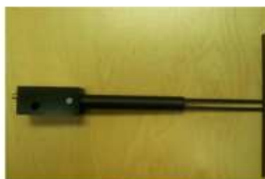
Figure 1 – MVG COMOSAR Validation Dipole
