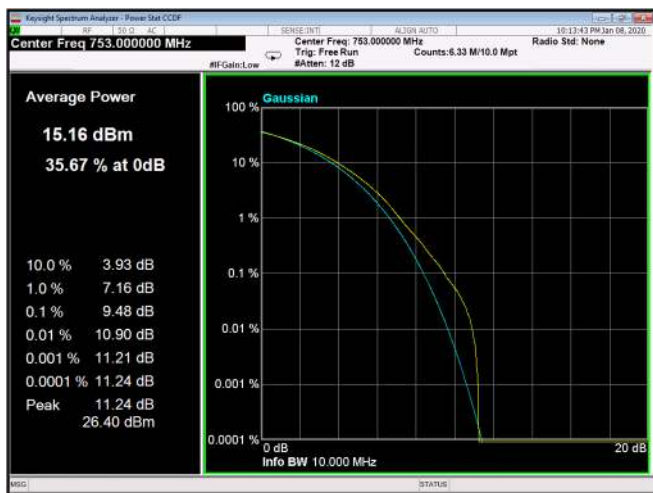
Figure 336: QPSK 10MHz B.W.; 753.0MHz, 15kHz
