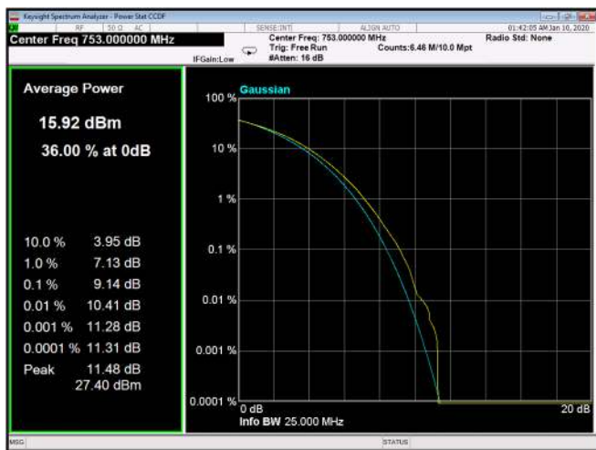
Figure 270: 64QAM 10MHz B.W.; 753.0MHz, 15kHz
