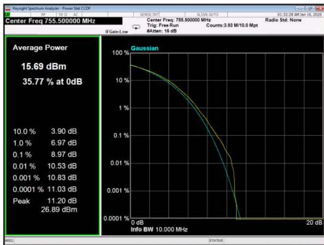
Figure 262: 64QAM 5MHz B.W.; 755.5MHz, 15kHz
