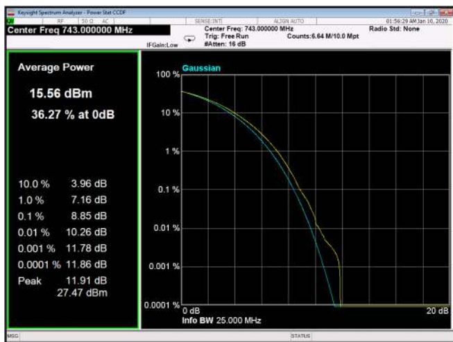
Figure 276: 64QAM 15MHz B.W.; 743.0MHz, 15kHz
