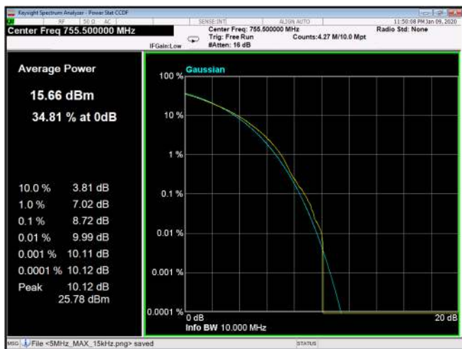
Figure 296: 256QAM 5MHz B.W.; 755.5MHz, 30kHz
