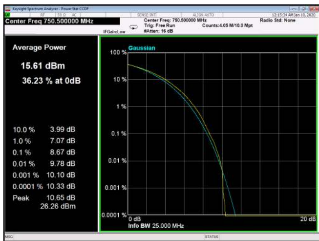
Figure 312: 256QAM 15MHz B.W.; 750.5MHz, 15kHz
