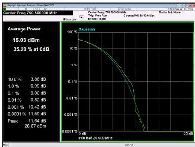
Figure 314: 256QAM 15MHz B.W.; 750.5MHz, 60kHz
