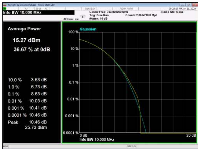
Figure 234: 16QAM 10MHz B.W.; 753.0MHz, 15kHz
