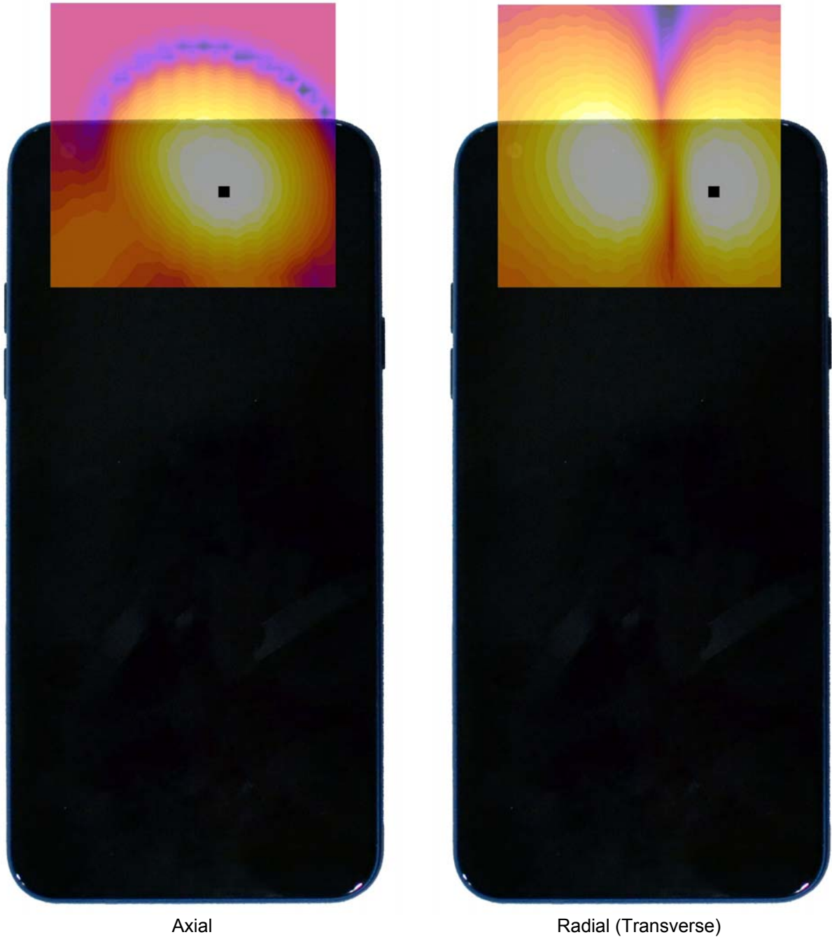
Figure 16-3 T-Coil Scan Overlay Magnetic Field Distributions
