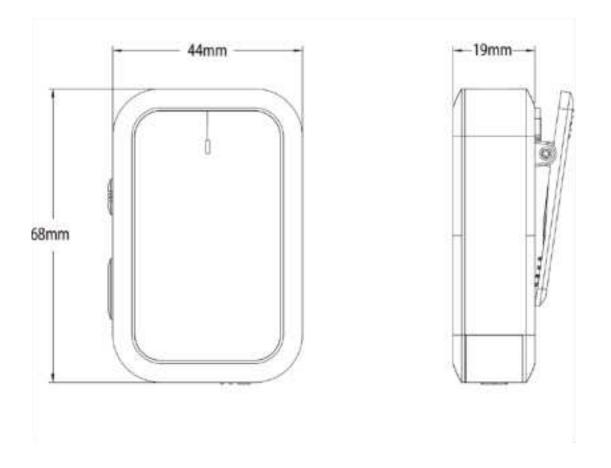
Product specifications 2xAAA batteries (not included) x 3 devices Directivity: Cardioid Sensitivity:-30dB±3dB Output impedance:≥2.2K Channel qty:20CH Transmit power:≥10dB Max Frequency Deviation: ±10KHZ SNR:≥81dB
