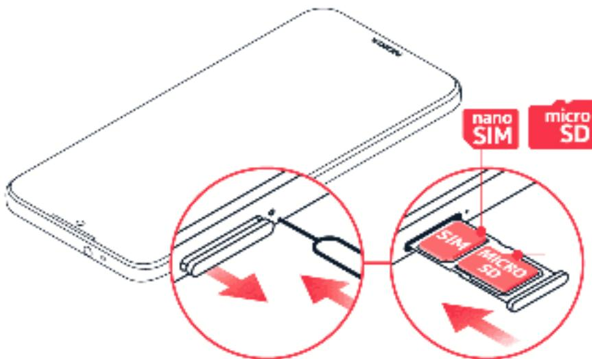
1. Open the SIM card tray: push the tray opener pin in the tray hole and slide the tray out.
