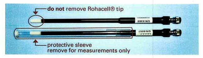
Note that probe usage is limited to free-space measurements; water, sugar-water solutions, nutrient solutions and glycol solutions will permanently damage the probe.
