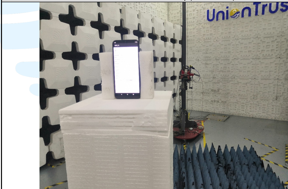
Radiated emission Test Setup (Above 1 GHz)
