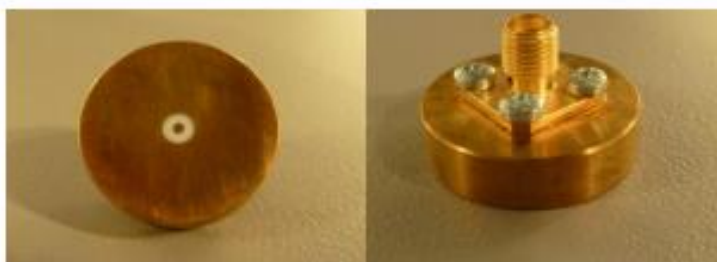
Figure 1 – MVG LIMESAR Dielectric Probe
