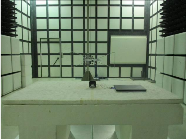
FCC 15 247 BLE Radiated Setup
