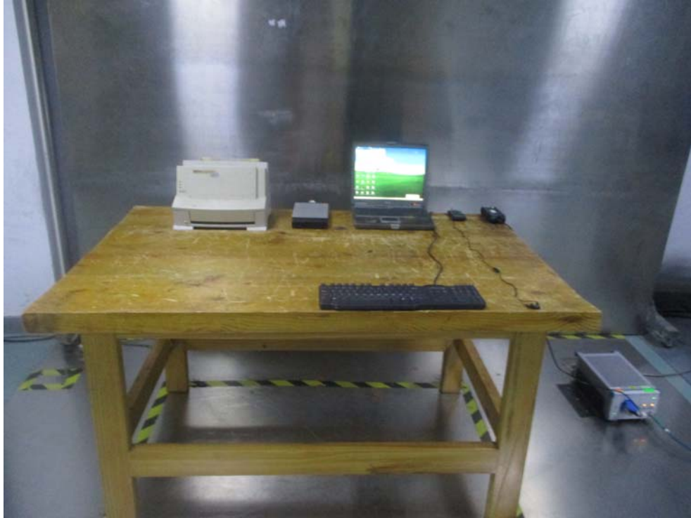
Conducted Emissions – Side View
