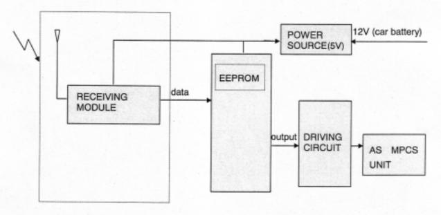
Figure 3.1 block diagram of the receiver
