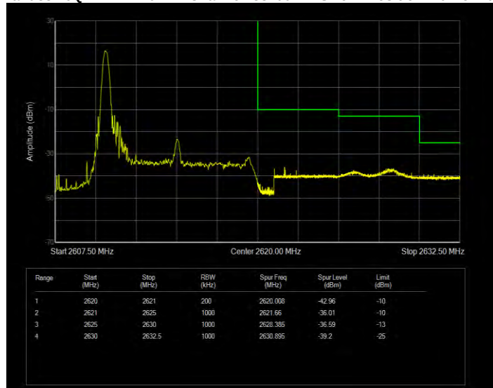
Band38 16QAM BW=10MHz Channel=38200 RB Size=1 Position=#Max Extended
