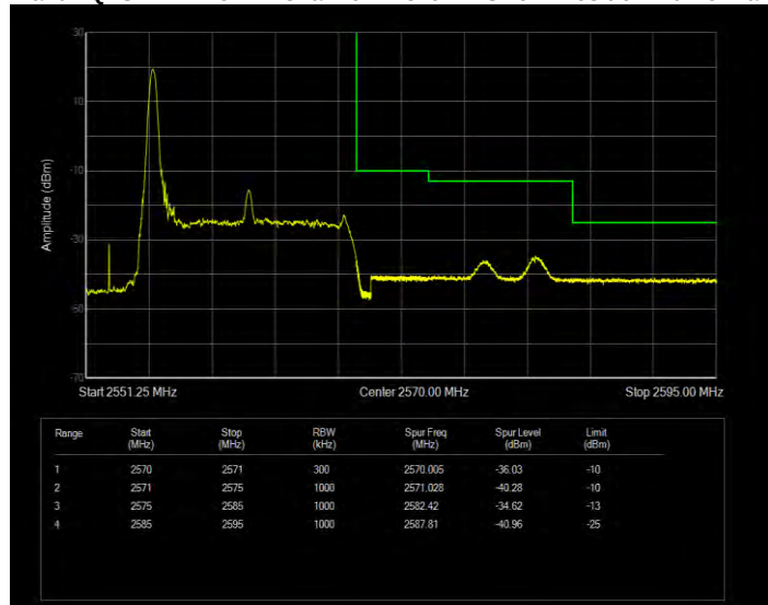
Band7 QPSK BW=15MHz Channel=21375 RB Size=1 Position=#Max Extended
