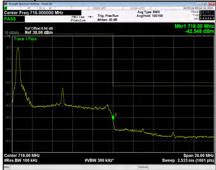
Band17 16QAM BW=10MHz Channel=23800 RB Size=1 Position=#Max Extended
