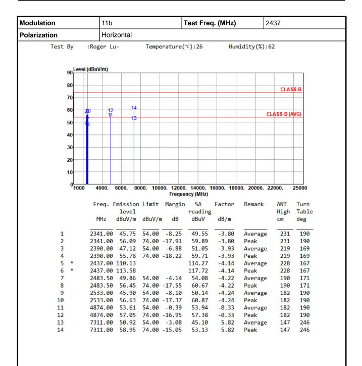
\*Factor includes antenna factor, cable loss and amplifier gain
