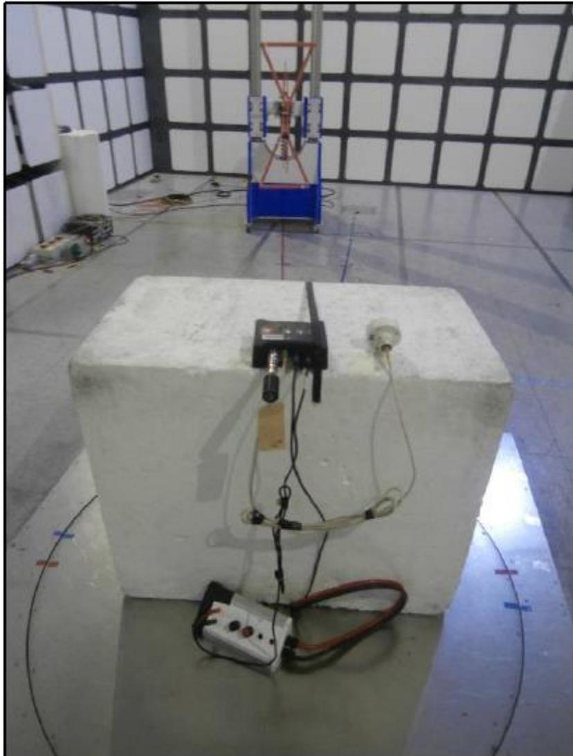
Figure 1 – 30 MHz to 1 GHz, EUT Orientation X
