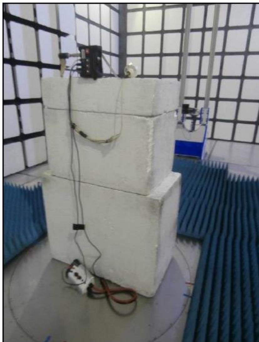
Figure 6: 1GHz to 2 GHz EUT Orientation Z
