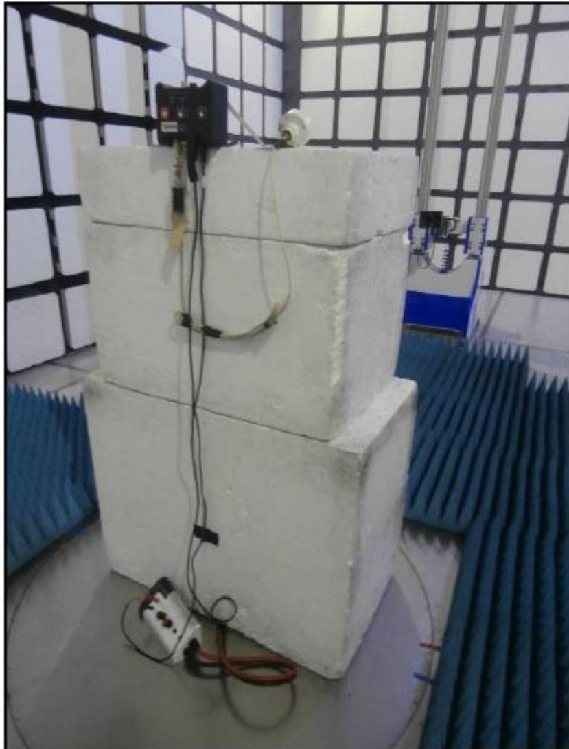
Figure 4: 1 GHz to 2 GHz EUT Orientation Y
