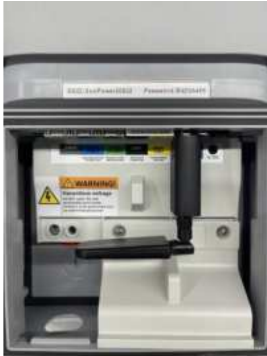
Photo 2.1: The communication module in the measurement meter
