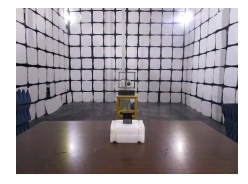
Spurious Radiation Test Setup (9kHz to 30MHz)
