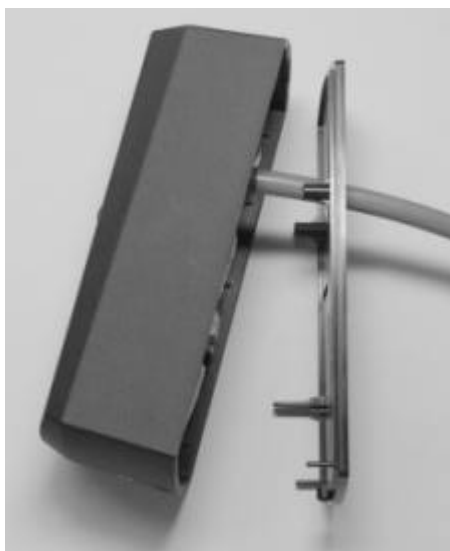
Figure 5> Separating the case
