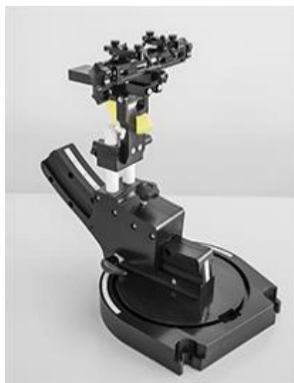
A simple but effective and easy-to-use extension for the Mounting Device; facilitates testing of larger devices according to IEC 62209-2 (e.g., laptops, cameras, etc.); lightweight and fits easily on the upper part of the Mounting Device in place of the phone positioner. The extension is fully compatible with the Twin SAM, ELI and other Flat Phantoms.
