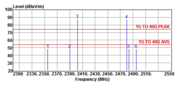
Site :CHAMBER #2 Date : 2017-03-24 Limit :1G TO 40G PEAK Ant. Pol. :VERTICAL **EUT** : BRYDGE 12.3" Model : BRY7201 :DC 5 V From NB :22°C **Power Rating** Temp.
