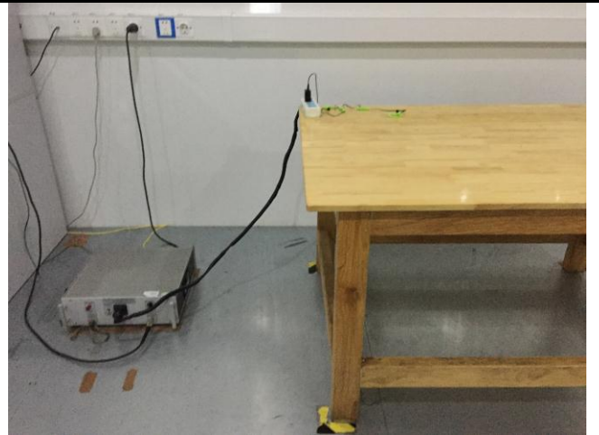
Conducted Emissions Test Setup Side View
