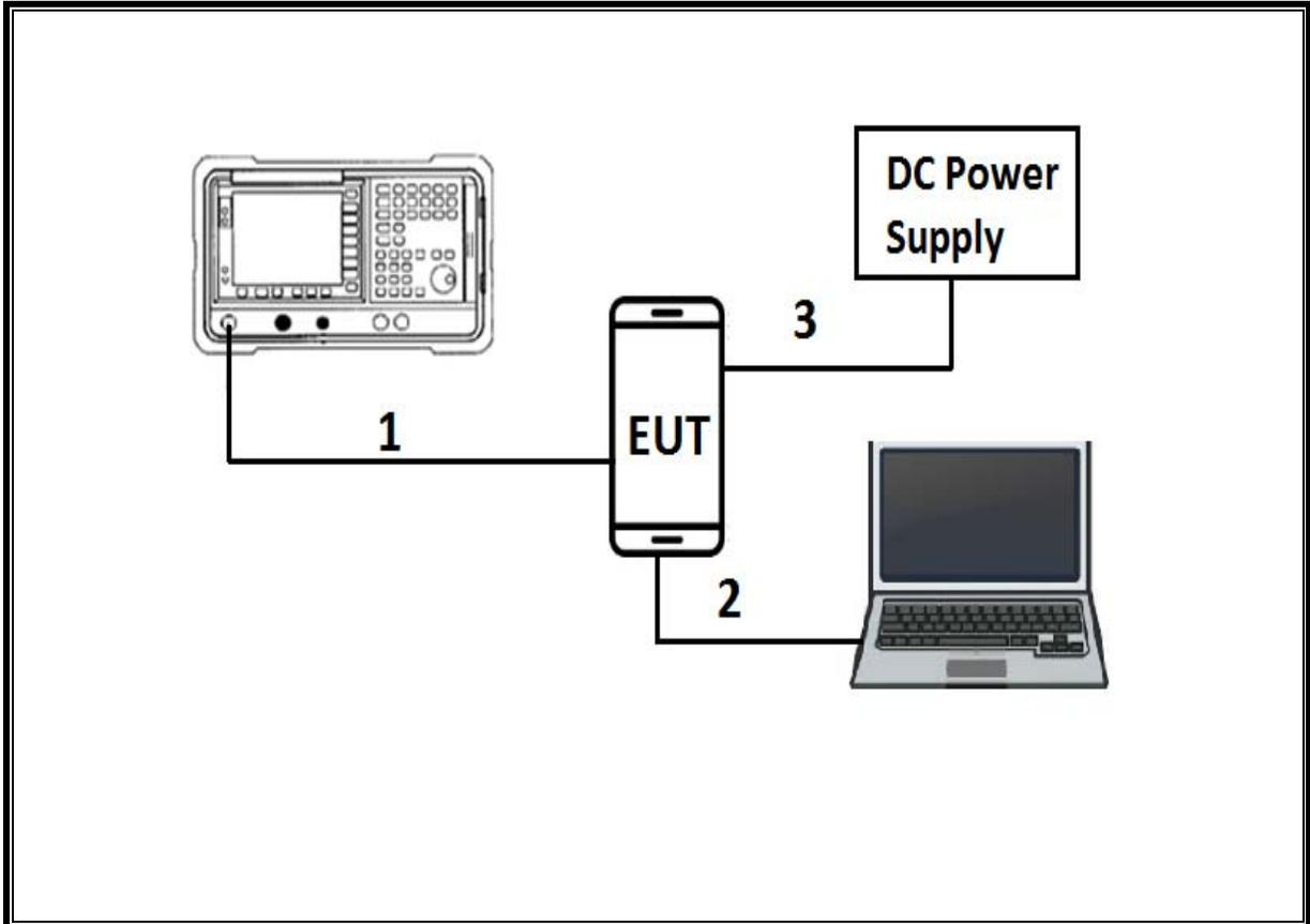
**TEST SETUP- RADIATED-ABOVE 1 GHZ and AC LINE CONDUCTED TESTS**
