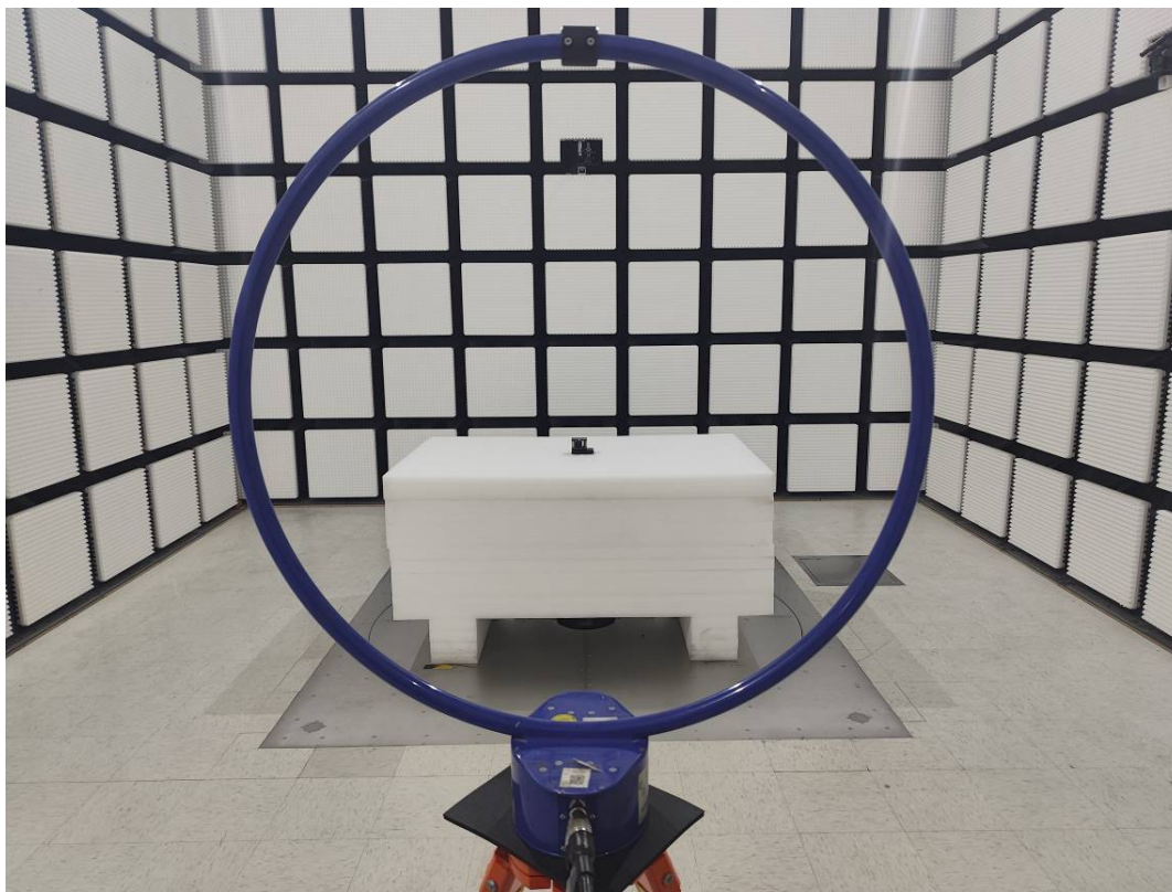
Radiated Emission 9k-30MHz Perpendicular View-M3
