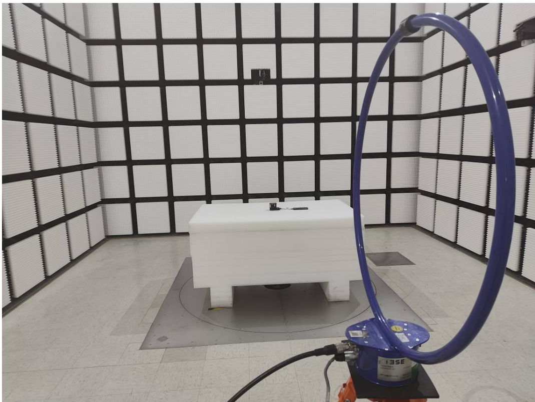
Radiated Emission 9k-30MHz Perpendicular View-M2
