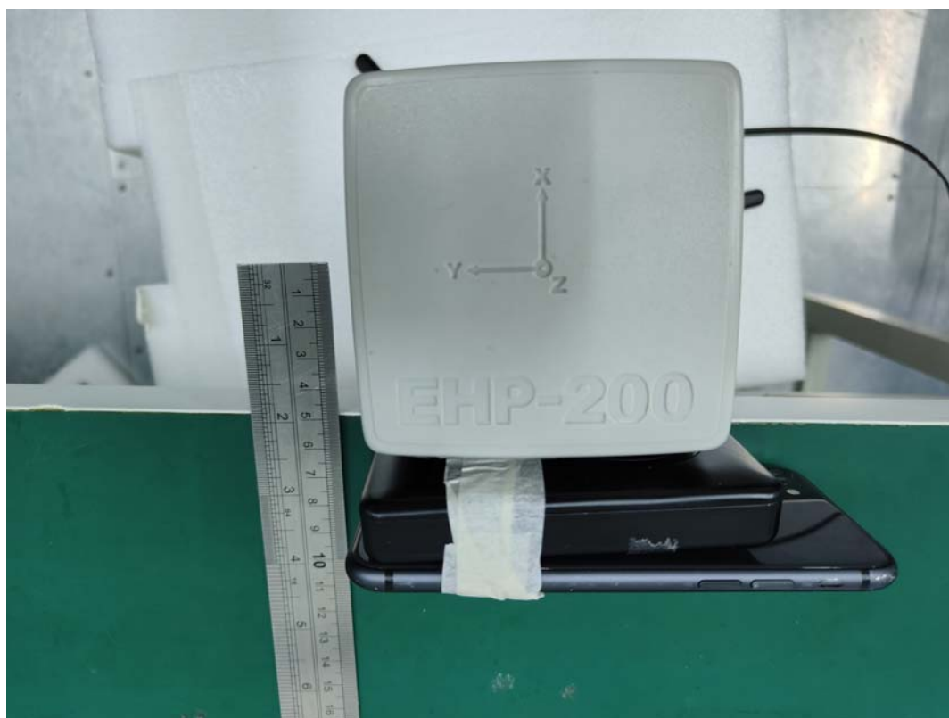
H-Field Position F Test distance 0-4cm M3
