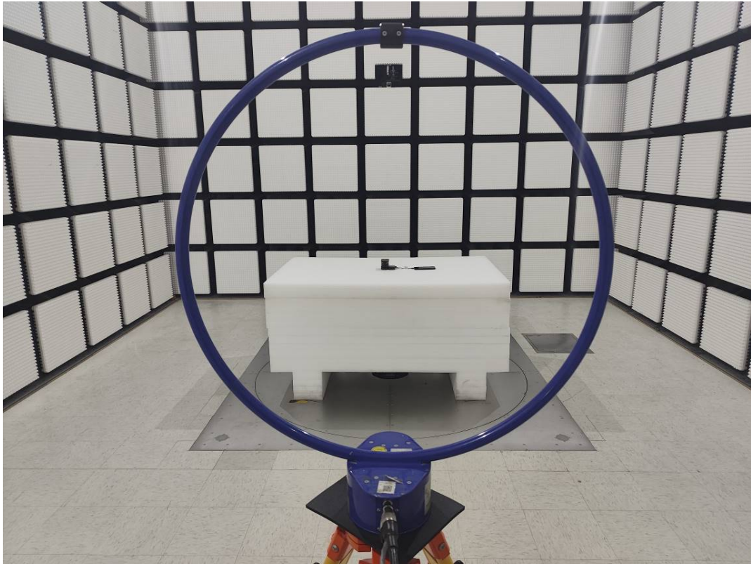
Radiated Emission 9k-30MHz Perpendicular View-M2
