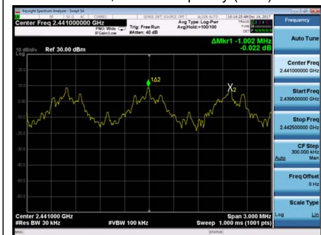
BT 3DH5 CH39, Carrier frequency (MHz): 2441
