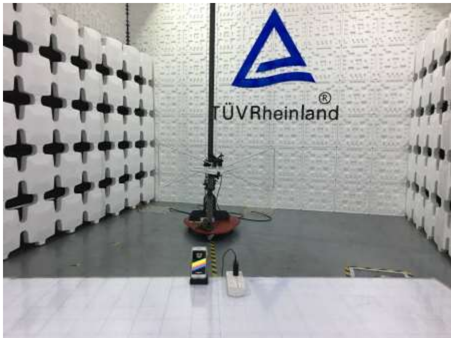
Photograph 2: Set-up photo for Radiated Emission, 30MHz - 1GHz
