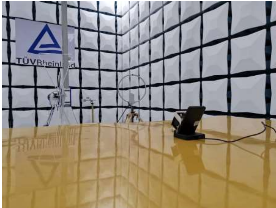
Photograph 1: Set-up photo for Radiated Emission, 9KHz - 30MHz
