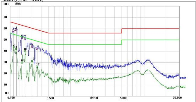
EUT: **Portable Wireless Speaker** Phase: L1 M/N.: BTS13 **Temperature:** 26°C 3-DH5 2402MHz **Humidity:** 54%RH Mode: **Test Engineer: Power Rating:** AC120V/60Hz Aiden
