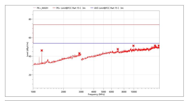
EUT: **Portable Wireless Speaker** Temperature: 24.5℃ M/N.: BTS13 **Humidity:** 55%RH Power Rating: Mode: 3-DH5 2480MHz **DC 3.7V Test Time: Test Engineer:** 2023-08-03 **Berny**
