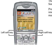
There are two soft keys on the two sides of your Smartphone, located directly below the display screen.
