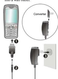
**3.** The status indicator on the Smartphone glows orange to indicate that battery charging is in progress. The indicator is off when the battery is fully charged.
