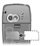
To install the battery, insert the two projecting parts on the battery into the holes in the battery compartment, and then close the battery. You should hear a "click" sound when the battery lock is engaged.
