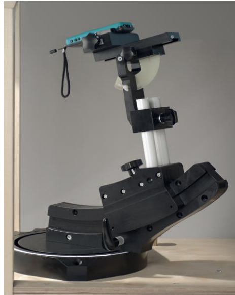
F-2. Device Holder for Transmitters
