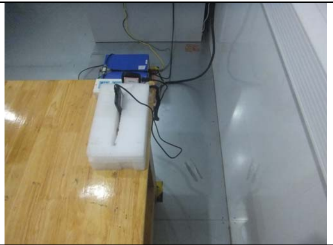
Conducted Emissions Test Setup Side View
