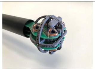
Test probe, without the casing
