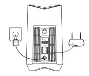
${f D}$  Turn on the H ${f H}$  HomeStation and connect it to your router. When the LED light turns blue, it means the H ${f H}$  HomeStation is ready for setup (this will take approximately 1 minute).
