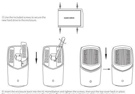
You can expand your storage room after cutting off power to the HomeStation by following the steps above The new hard drive must be initialized through the Baseus Security APP for use with the H1 HomeStation
