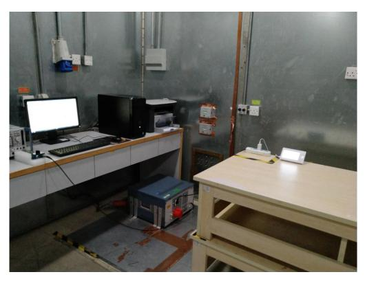
RADIATED EMISSION TEST SETUP BELOW 1GHZ
