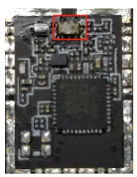
3. U3418=VC1618A SP8T Switch main function: WCDMA/LTE diversity receiving antenna switch
