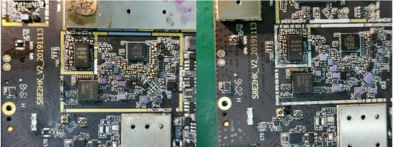
2, U3916=SLFT21-2R450G-02T Triplexer for GPS&WIFI (2.4G/1.57G/5G) Main function: 2.4G/1.57G/5G power splitter
