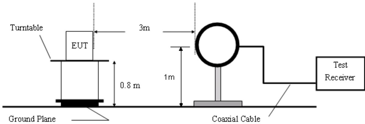
Figure 1. 9KHz to 30MHz radiated emissions test configuration
