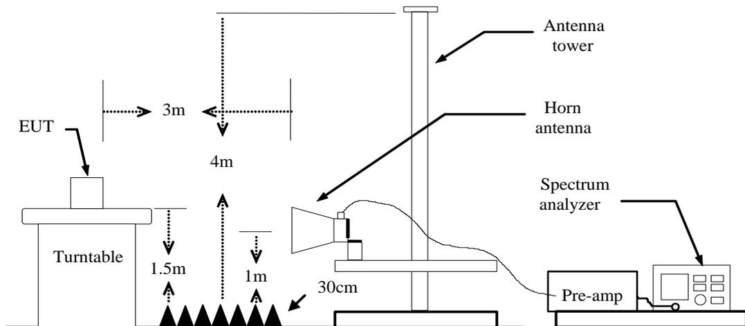
Figure 3. Above 1GHz radiated emissions test configuration
